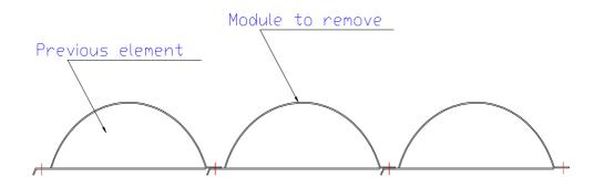
Using a lever, slightly lift the previous element and place a thickness of wood (5 cm) between the panel and the tank edge to facilitate the extraction of the module to be removed (see figure).
